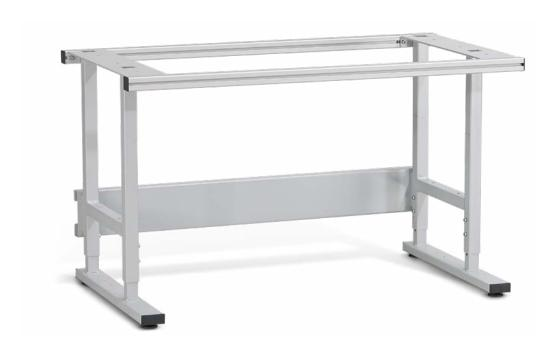
Robust design made of  $40 \times 40$  mm tubular steel combined with a sturdy rear C-profile to support the addon units.  $40 \times 40$  mm aluminium profile sections are used at the top to hold the worktops and for securing the drawers. High-quality powder coating in RAL 9006 white aluminium.
