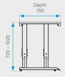
The ERGO-Vario Plus basic frame is the ideal solution for standing/sitting workstations. Thanks to a high-quality guide rail, the table is also very strong and stable with the height fully extended. The table is fitted with an adjustment range of 300 mm as standard. This can be extended to
