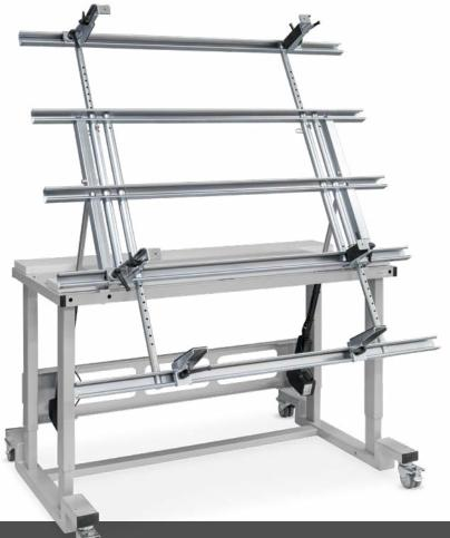
The ERGO-Mont is used for the assembly of control cabinets and mounting plates. Continuous adjustment of the height and inclination by means of an electric motor enables an ergonomic working position. Side brackets, which can be adjusted without tools, enable the simple fixing of the workpieces.
