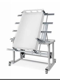
The ERGO-Mont base frame consists of a solid steel tube construction and four height-adjustable linear units, which can be height-adjusted by 500 mm via an electric motor. The inclination of the worktop can also be adjusted via an electric motor. A telescopic base frame and a flexible mounting system with side brackets facilitate the fixing of mounting plates and control cabinets.
