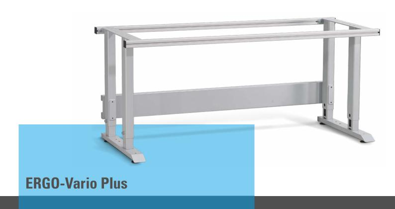
Robust design made of 80 x 50 mm tubular steel combined with a sturdy rear C-profile to support the add-on units. 40 x 40 mm aluminium profile sections are used at the top to hold the worktops and for securing the drawers. High-quality powder coating in RAL 9006 white aluminium.
