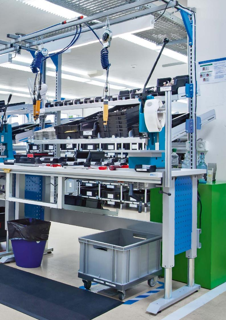
Free-standing add-on units offer a cost-effective alternative to a table. E.g. when the conveyor equipment already exists and you simply want to incorporate a packing process. Different grid widths can be combined with other as needed.
