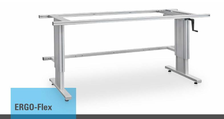
Stable structure comprising the lateral aluminium guides, which are connected via a sturdy crossbeam. 40 x 40 mm aluminium profile sections are used at the top to hold the worktops and for securing the drawers. High-quality powder coating in RAL 9006 white aluminium.
